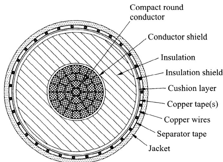
*Cross section of solid-dielectric power cable with concentric wire shield*
